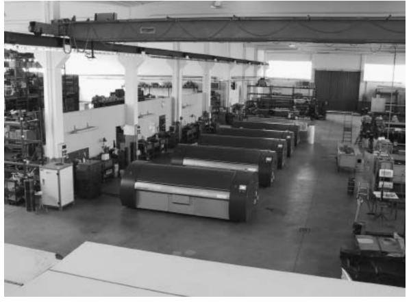
The Creo/Acigraf Exactus system, showing the different units that are used for all the stages of processing. These include coating, imaging, developing, mask removal and finishing. The cylinder might then also move to a further chroming process.
