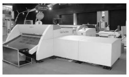
The Screen PlateRite Ultima 32000 images plates from 4-up to 32-up, with one GLV exposure head up to 30 8-up plates per hour. With two GIV heads, it is named Ultima 32000Z and images simultaneously up to 46 plates 8-up plates per hour or 22 212.4by-127.6-cm plates per hour.
