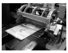
A.B.Dick's chemical free Vector CTP system with the "thin drum."
